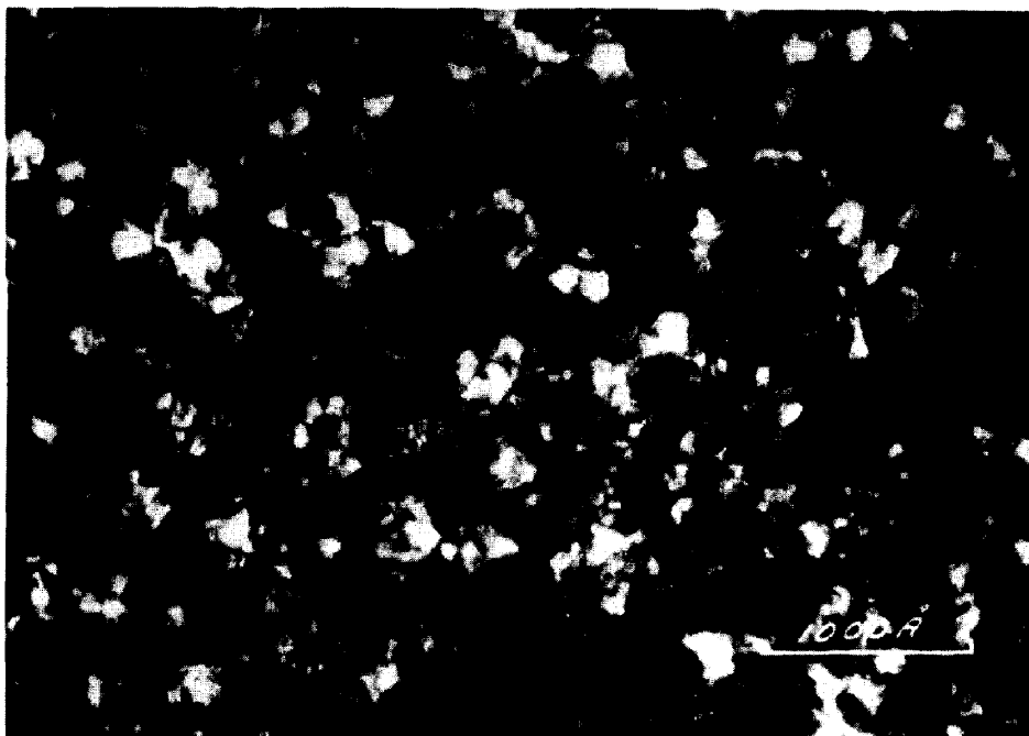
FIG. 13. Tungsten, condensed on substrate at 670°K.
